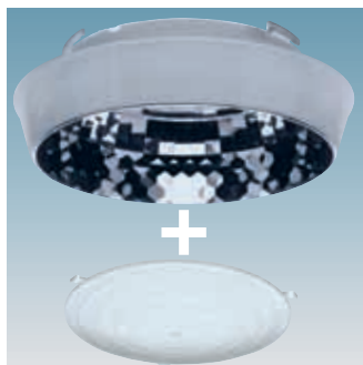
Diffuser transp. 91810 Baffle in transparent, self-extinguishing polycarbonate material with prismatic faceting and silking for great glare control. To be bought with acc. 91805. Only FLC1x18D and FLC2x18D.
