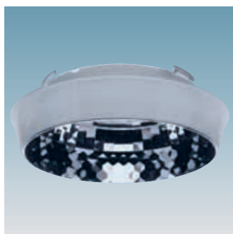
Facetted ring 91805 Low luminance "dark light" ring 65° (EN 12464). In metallic polycarbonate with prismatic faceting for greater light control.
